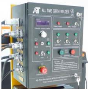
Master control panel integrated with Lincoln NA3 welding control
